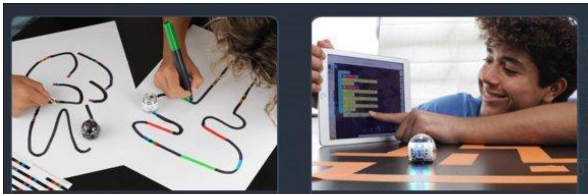
Figure 8: lines with colour codes (left) and ozobot with programming environment (right) (picture from Ozobot & Evolve, Inc. United States 2020)
