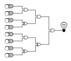
The output from the component  $\xrightarrow{=}$  is ON only when BOTH incoming wires are ON.
